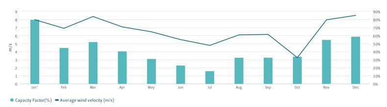
Wind velocity is relatively high, at a relatively low height in Iceland. This significantly reduces the cost of energy and operating costs as hub heights can be kept much lower than in other countries.
